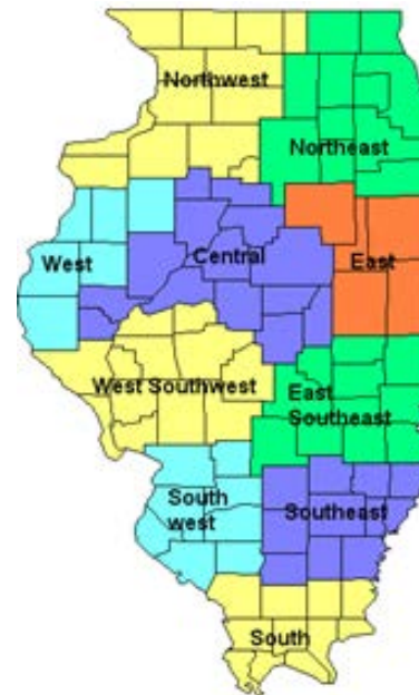
Figure 60: Map excerpt from Bulletin 70 which illustrates the 10 rainfall frequency sections in Illinois ( http://www.isws.illinois.edu/atmos/statecli/RF/fig1-rf.gif )
